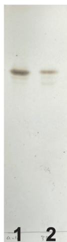
Fig. 4. Thin-layer chromatogram of mussels-derived ceramide 2-aminoethylphosphonate Lane 1, mussels-derived ceramide 2-aminoethylphosphonate; lane 2, standard ceramide aminoethylphosphonate. The plate was developed in chloroform/methanol/water (60:30:5, v/v/v) and the spots were visualized with 50% (v/v) sulfuric acid solution.
